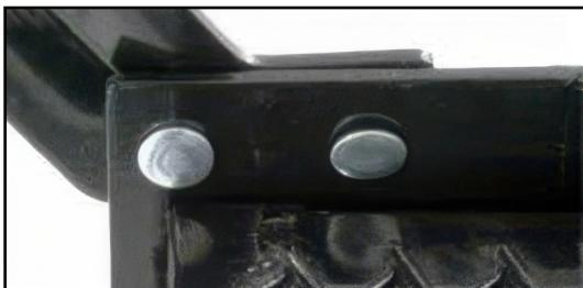
**NOTE:** Fully tighten the carriage bolts only after the ramp is in the upright position and the spring pins are locked into place. This will align the pins with the holes in the ramp as there is some play in the bracket that could cause misalignment if this procedure is not followed.
