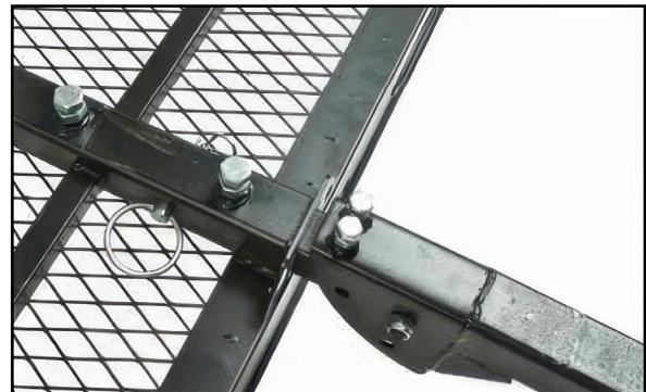
**STEP 3.** Flip the carrier right side up and install the ramp bracket (B) using the carriage bolt sets (D) using a 13mm or 1/2" wrench. Be sure the square shoulders on the carriage bolts seat fully in the square holes on the carrier.
