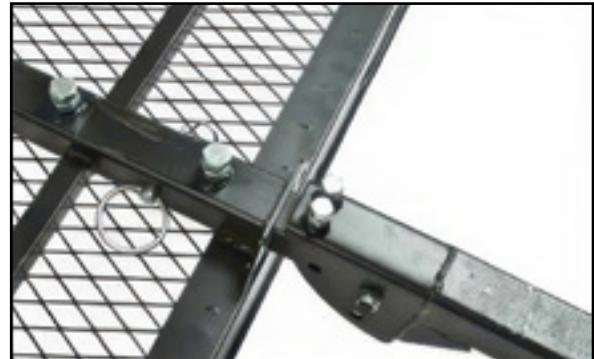
**STEP 3.** Flip the carrier right side up and install the ramp bracket (B) using the carriage bolt sets (D) using a 13mm or 1/2" wrench. Be sure the square shoulders on the carriage bolds seat fully in the square holes on the carrier.
