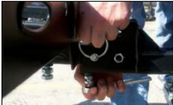
Remove the pin with clip (J) to fold the carrier vertically. Replace the pin in the top pin hole to secure the carrier in the vertical position.
