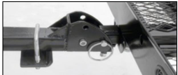
**STEP 7.** Securely tighten the hex head pivot bolt on the hitch tube assembly with a 10mm Allen wrench to eliminate side-to-side wobble of the hitch carrier. If the bolt is not properly tightened, it may cause the carrier to not be level.
