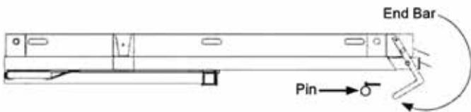
**Step 2.** With both pins pulled from the carrier, pull the loading deck out.
