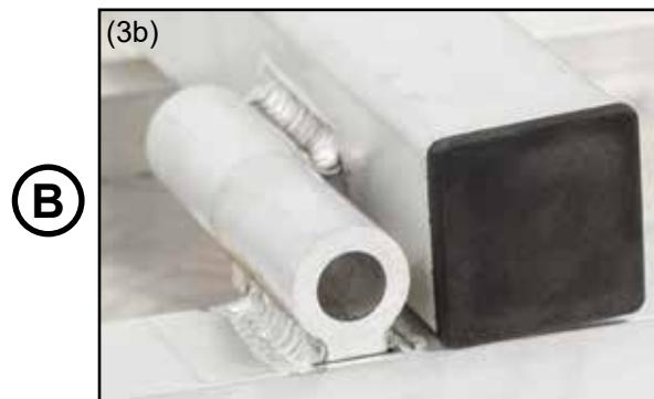
**Step 4.** Make sure the hinges are aligned and insert a Straight Hitch Pin (5) through the hinges from the inside out. Secure with a Cotter Pin (6). Repeat with the other side. The Cotter Pin will be on the outside of the Carrier Deck, NOT underneath for both sides.
