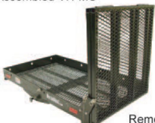
Note: the Ramp is being held in the upright position by the Spring Pull Pins on the Ramp Bracket.
